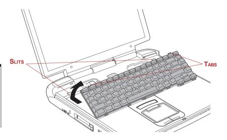
Figure 8-9 Removing the keyboard (2)
